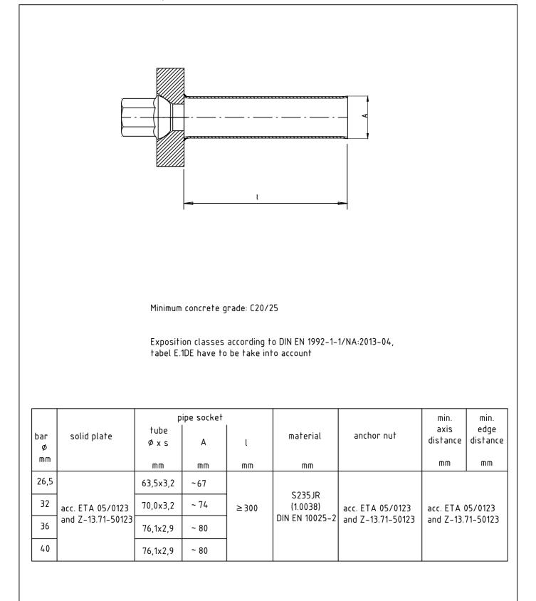
Permanent DYWIDAG Anchors (Single Bar Anchors) for Soil and Rock with steel tendons made of: St 950/1050 Ø26,5mm,Ø32,0 mm,Ø36,0 mm und Ø40 mm
